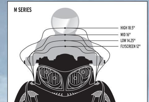
NOTE: MEASUREMENTS ARE TAKEN VERTICALLY FROM DASH PANEL TO TOP OF WINDSCREEN
